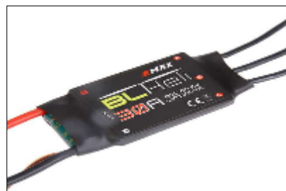
Figure 7 Electronic Speed Controller
