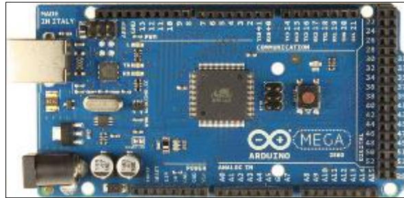
Figure 5 Arduino Mega 2560 R3
